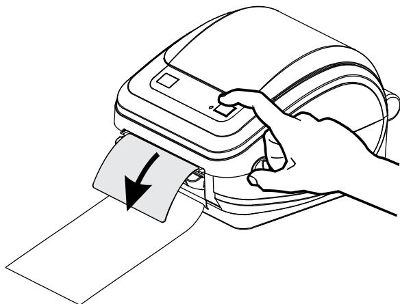
6. During the print job, the printer will peel off the backing and present a single label. Taking the label from the printer to allow the printer to print the next label. Note: If you did not activate the label taken sensor to detect the removal of the dispensed (peeled) label with software commands, the printer will stack and eject peeled labels.
