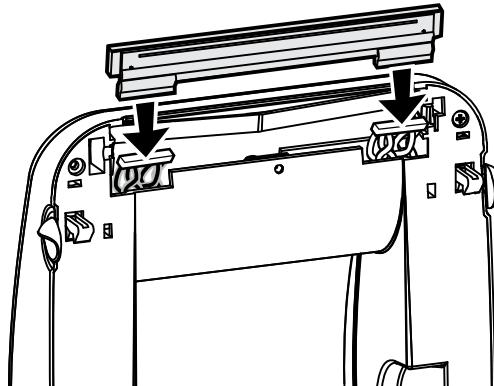
2. Slide the printhead into the left side and jog it into the right side catch.
