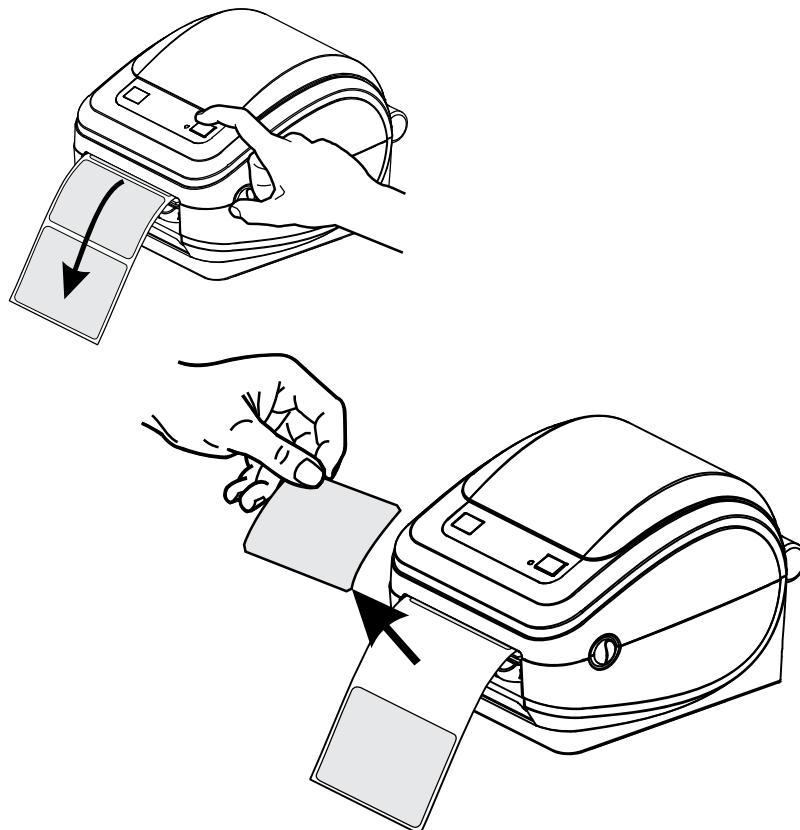
2. Lift the liner over the top of the printer and open the dispenser door.
