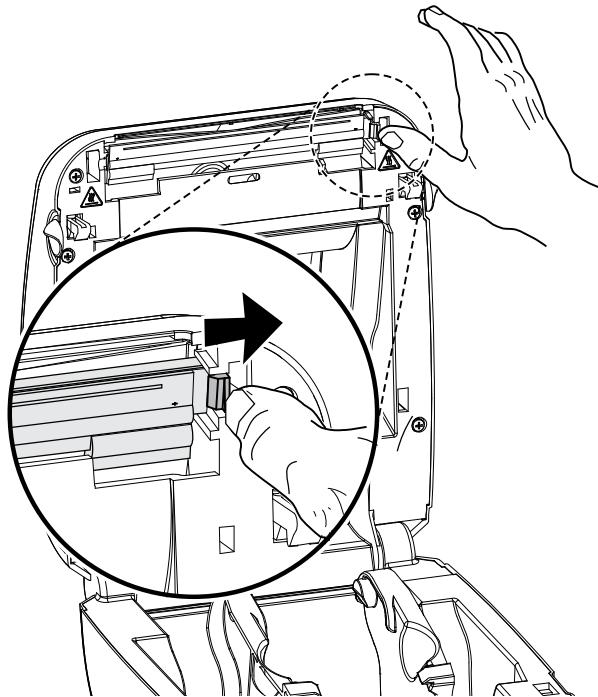
2. Pull the printhead forward and pull it free of the top case if necessary.
