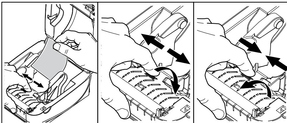
**3.** Insert the media through the slot at the rear of the printer.
