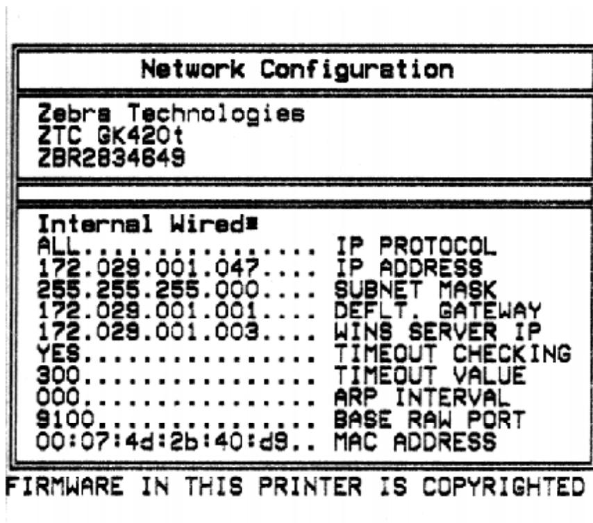
The regular printout of the configuration status label has some of the printer's network settings such as IP Address, on the lower half of the printout.
