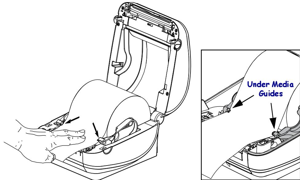
5. Close the printer. Press down until the cover snaps closed.
