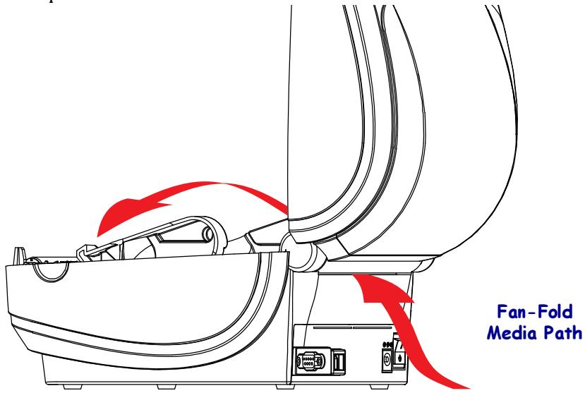
2. Adjust the media guide stop position with the green thumb wheel. Use a piece of the fan-fold media to set the stop position. Rotate the wheel away from you to open the guides wider. Rotate the wheel towards you to make the media guide narrower.
