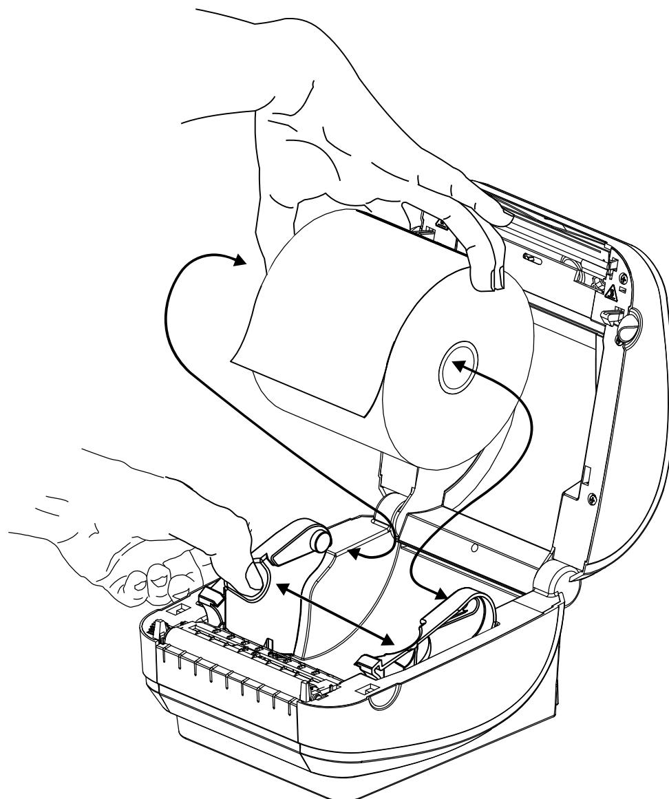
3. Pull the media so that it extends out of the front of the printer. Verify the roll turns freely. The roll must not sit in the bottom of the media compartment. Verify that media's printing surface is facing up.
