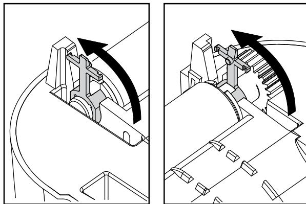
3. Lift the platen out of the printer's bottom frame.
