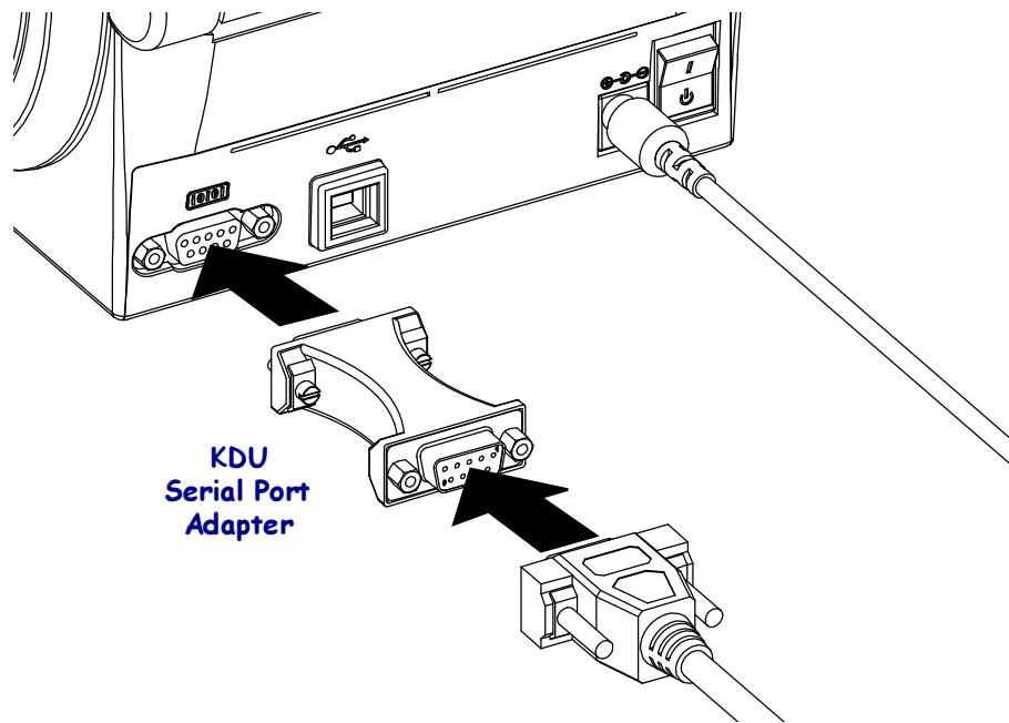
3. Plug the adapter onto the printer's serial interface; use a small, slotted screwdriver to tighten the screws and secure the adapter.
